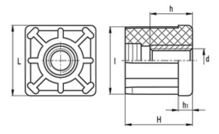
$\begin{array}{lll} d & = M16 \\ h & = 15 \\ H & = 45 \\ h1 & = 10 \\ Internal tube size = 47.6 \\ I & = 47.6 \\ L & = 50 \\ \end{array}$
